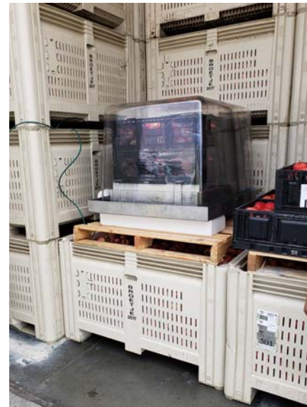
SafePod in Position in Doorway of CA Room
